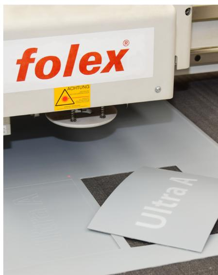
In contrast to many rubber-based coating blankets, the compressible element is attached under the polyester carrier. It is thus protected against penetration by washing agents or coatings and can be used multiple times. Water-based and UV coatings can be processed perfectly. In the usual way, coating forms can be produced quickly and hassle-free.
